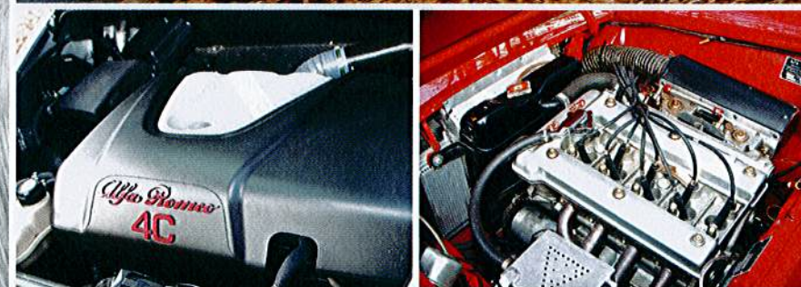
4C's turbo 1.7-litre four has 237bhp; GTA's 1.6 twin-cam makes 160bhp here, not the stock 115bhp
