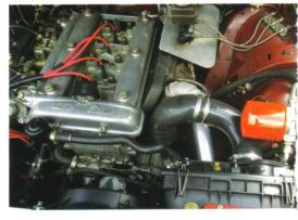
Engine bay with neat installation work. Braided brake pipes and modern silicone plumbing have been added by Mike Spenceley.
